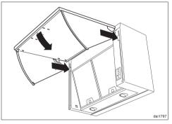
Position the vapour canopy with the cabinet front fitted and close it.
